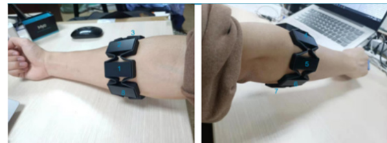
Figure 2. MYO ring acquisition signal schematic. The 7 hand gestures include fist grip, holding a cellphone, palm-to-palm exercise (cupping), cylindrical grip (holding a water cup), finger opposition exercise (thumb and index finger gripping a pen), single finger extension (extending index finger to touch the screen), and lateral thumb pinch (pinching a key, etc.) (as shown in Figure 3(a)). The multimodal signals include 8-channel sEMG signal, 3-channel arm acceleration signal, 3-channel angular velocity signal, 4-channel quaternion signal. Acceleration, angular velocity, and quaternion are inertial measurement units (IMU).
